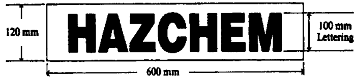
Figure 2 — Template for a placard for dangerous goods (other than C1 combustible liquids) in bulk
